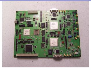
The PCI-DSP-FPGA series of boards provide advanced capabilities of using both DSPs and FPGAs enabling a variety of sequential and parallel processing tasks to be integrated in truly real-time operation. These boards provide enhanced functionalities over the PCI-DSP series.
