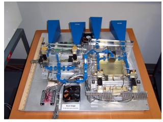
Each radar unit has two receiving and two transmitting channels with different (vertical or horizontal) polarizations. The transmitters can be alternated at each IPP or after any selected number of IPPs. The receiver channels (V and H) always operate for each IPP.
