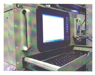
The Real Time Signal Intercept, Analysis and Countermeasure system provides an integrated system to capture wide band RF signals, perform real time analysis of the signal, and if necessary, take effective countermeasure. It performs most cognitive radio functions necessary for communication, navigation and radar surveillance, intercept, analysis, and countermeasure.
